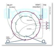
For the oxygenates channel the system can be configured with a so-called Deans switch. A pre-separation is made on the methyl-silicone pre-column. The oxygenated components are cut from the matrix by applying a pressure switch, directing the effluent from the pre-column either to the monitor column (vent) or to the analysis column. This concept ensures that there is no co-elution of the matrix with any of the oxygenates to be analyzed.
