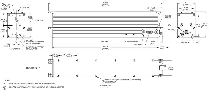
3 LASER IS MOUNTED BY REMOVING COVER SCREWS AND REPLACING WITH APPROPRIATE LENGTH SCREWS FOR YOUR MOUNTING APPLICATION. USE A MINIMUM OF FOUR SCREWS IN A SYMMETRICAL PATTERN TO PROPERLY DISTRIBUTE MOUNTING FORCES. DO NOT REMOVE COVER.
