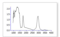
A typical IR spectrum from FluidScan
