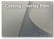
Multiple wavelength options and excellent peak power to cut polymer films with crisp edges and minimal lip melt, essential for modern electronics manufacturing.
