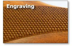
Stable operation over a wide range of settings enables precise control of material removal, allowing consistent ablation depth or detailed 3D engraving.
