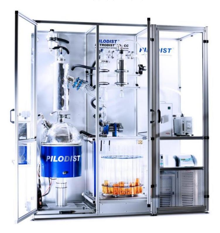
This new edition is summarizing our long term experience and taking into account all our customers feedbacks for improved performance and even more easy handling and reduced service necessity. The new design specifically highlights the high viscous residues that are being processed in this system by guaranteeing a continuously operating tempered discharge into an open fraction collector with automatic and precise weight measurement.
