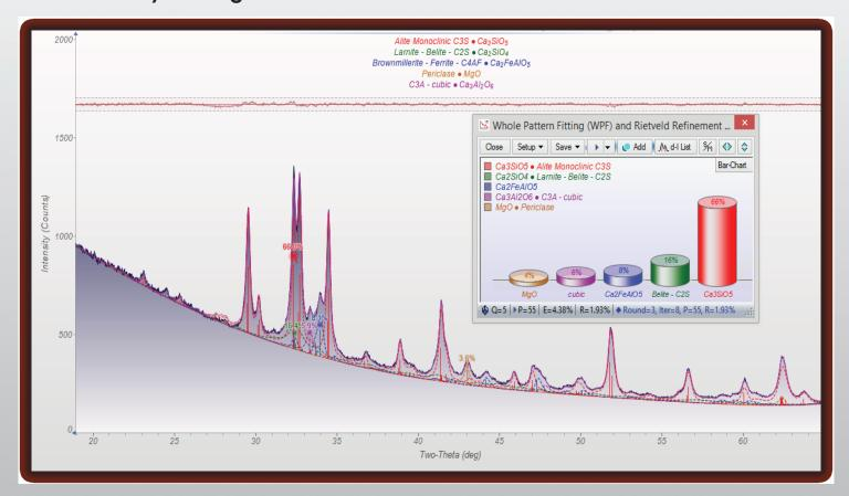
Through the use of our economical benchtop AXRD unit coupled with powerful JADE powder diffraction software one can perform quantitative phase analysis utilizing whole pattern fitting and Rietveld refinement to determine the composition of various types of raw feed materials to ensure optimal properties of the produced final product.
