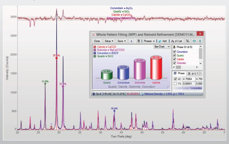
Through the use of our economical benchtop AXRD unit coupled with powerful JADE XRD analysis software one can perform quantitative phase analysis utilizing Rietveld refinement to determine the composition of various types of corrosion and scale products.
