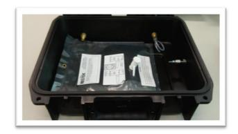
To prevent unsafe situations, the Gas Box Sampler is equipped with a pressure relief valve, which is adjusted to a pressure well below the limits of the box. In addition, the box is not completely leak tight, an increasing pressure will cause some leakage on the sealing on the lid of the box.
