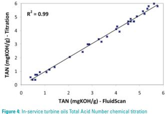
Figure 4: In-service turbine oils Total Acid Number chemical titration vs. FluidScan
