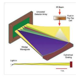
Figure 3: Patented wedged optical design
